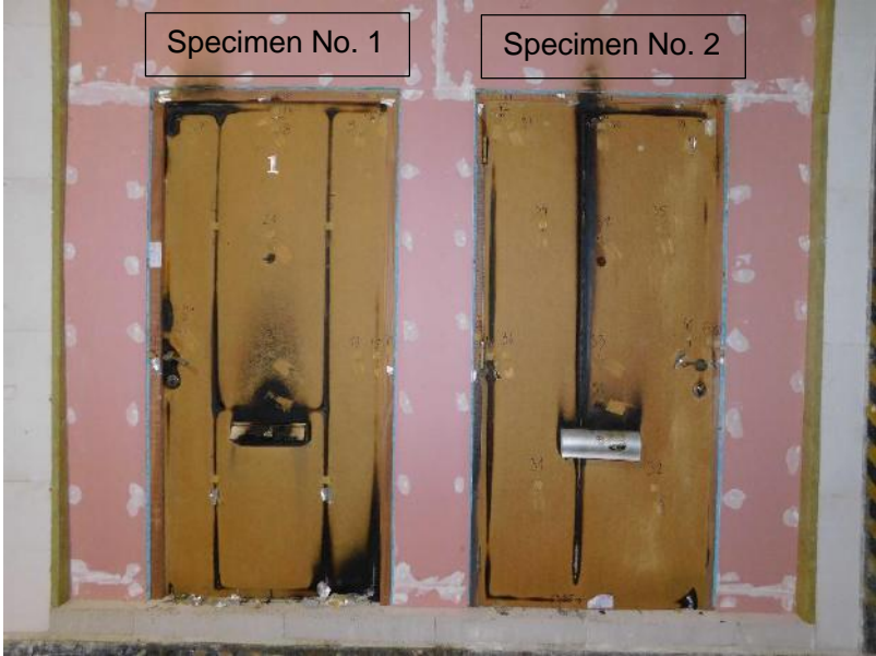
View of the unexposed specimens face after the termination of the test
