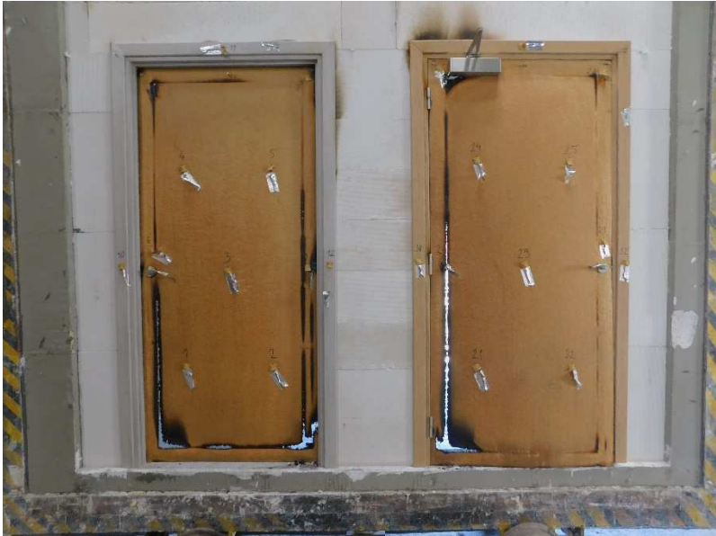
Unexposed specimen face after the termination of the test.
