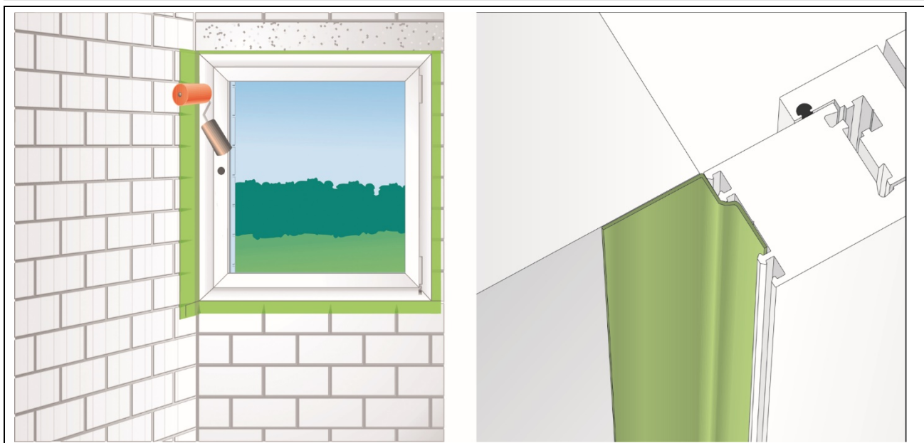
Figure 6 Installation of window and construction reveal material with the self-adhesive
