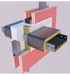
FB750 double batt with FI025 Intuflex: EI120 when tested with the EN cable set
