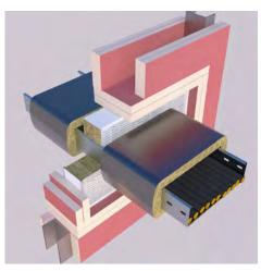
FB750 single batt with Fl025 Intuflex: El60 when tested with the EN cable set
