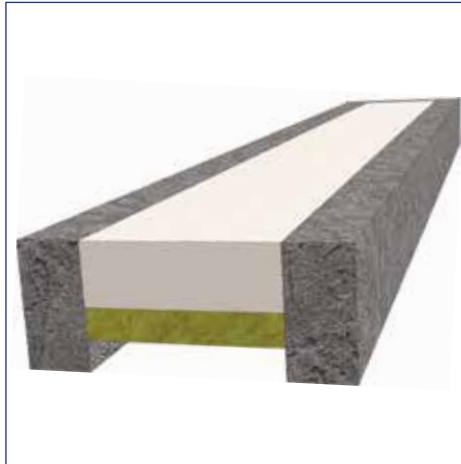
FR230 Intucompound + FI140 Shutter Slab for loadbearing unlimited lengths seals up to 300 mm width
