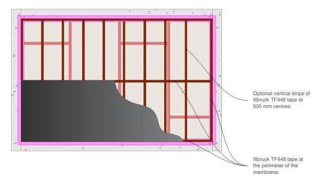
For low to medium wind loads the double sided tape should be applied around the entire perimter of the membrane. For higher wind loads, the bond can be further enhanced by installing vertical strips of TF448 High Performance Bonding Tape at 500 mm centres.
