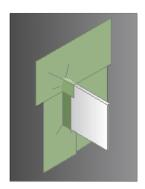
All incisions around any penetration are fully sealed with the correct illbruck tape.
