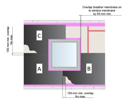
All overlaps are sealed with the correct illbruck tape, applied bubble and wrinkle free and the bond consolidated with a seam roller.
