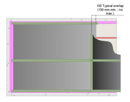
Once the joints have been formed and the membrane is secured, apply the correct illbruck tape to seal the overlaps. The applied tape should be wrinkle and bubble free, and consolidate with a seam roller to acheive the required bond strength.
