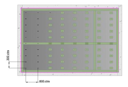
For other sheating boards and substrates types where staples are not suitable or where a greater resistance to wind loading is required, stainless steel screws are installed through the sheathing board into the SFS at 500 mm centres vertically and to align with every stud.
